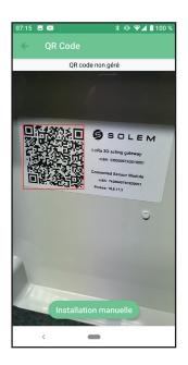
The «Manual Installation» mode allows you to install the Connected Irrigation Station in the event of a problem with scanning the QR code.
