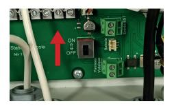
On start-up, the Station connects via the 3G / 4G network to the MySOLEM platform (provided you have requested activation of the SIM card using the document provided in the box of the Connected Irrigation Station). During this initialization phase, the LEDs inside the product will flash to indicate that the installation is in progress.
