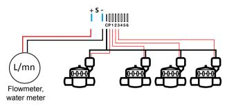
Connect your + S - input to a water meter equipped with a flow sensor as shown above. Use dry contact flow sensors or equivalent.
